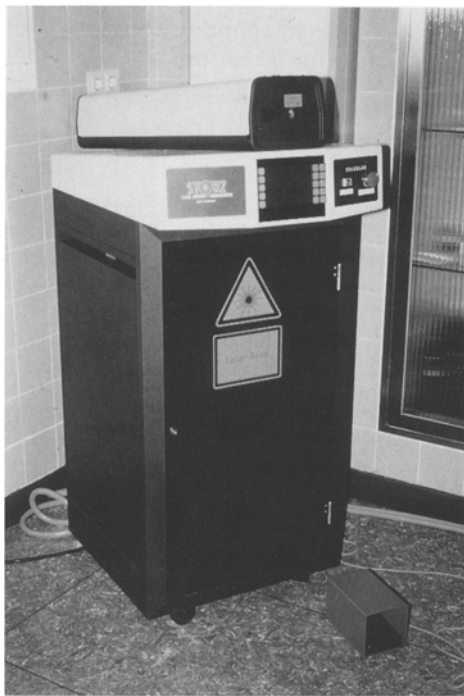
Fig. 6. Nd:YAG laser with three functions: nanosecond pulses for urinary stone disintegration and millisecond pulses for biliary stones and coagulation
